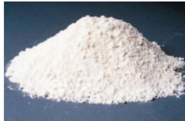
hardened concrete properties similar to industrial byproduct pozzolans. Some investigators have even reported that natural pozzolans are more effective in controlling alkali silica reaction than fly ash. More reactive pozzolans such as metakaolin and rice husk ash are often used in the same manner and proportions as silica fume.
