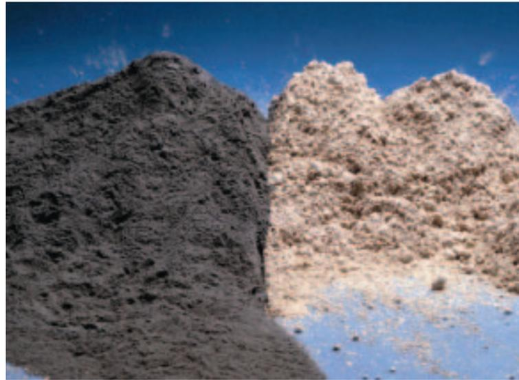
strength mix designs for such products as precast concrete bank vaults. Silica fume also can be used to increase the compressive strength of lightweight concrete as well as conventional concrete, making it possible to reduce the wall thickness or other dimensions of a product to overcome transportation limitations.
